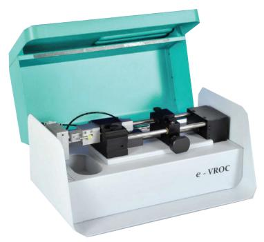
e-VROC™ provides extensional viscosity data by monitoring the sample flow through a microfluidic contraction within the measuring cell. The system measures the pressure upstream and downstream of a contraction using the MEMS pressure sensors, and it registers changes in the flow. The fluid undergoes an almost constant extension through the contraction/expansion, enabling the calculation of the extensional viscosity.
